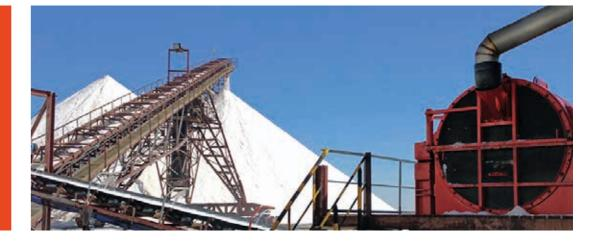
If the machine is too heavily loaded, the axial vibration The axial sensor enables the machine's loading condineeded for transport (originating from the "resonance" oscillator" design principle) is stopped, but overloading is not automatically identified and the machine goes on running. Also uneven loading, e.g. by using bucket loaders instead of screw conveyors, has been identified in various cause analyses as a reason for excessive radial deflection.
