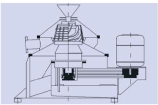
A number of design updates to vertical coal centrifuges failed to achieve ideal effect in terms of equipment overall performance, and the maintenance to it is very difficult. Now, all SIEBTECHNIK coal centrifuges adopt horizontal design, which is the state of the art technology, featured with large processing capacity and easy maintenance.
