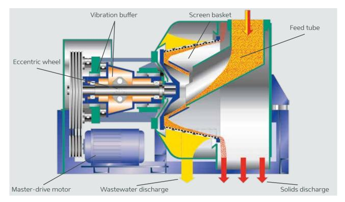
The well-designed horizontal vibratory screen centrifuge has high-efficient and high-yield performance. It is able to provide:
